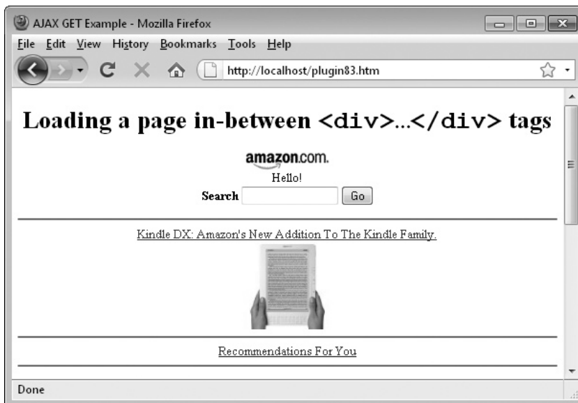
FIGURE 11-3 Ajax works equally well with either POST or (as shown here) GET requests.
