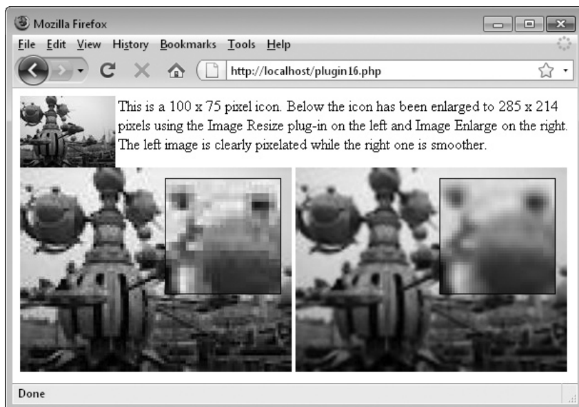
FIGURE 4-6 Even with resampling, enlarging a picture causes pixelation—but this plug-in helps reduce it, as shown by the zoomed-in insets.
