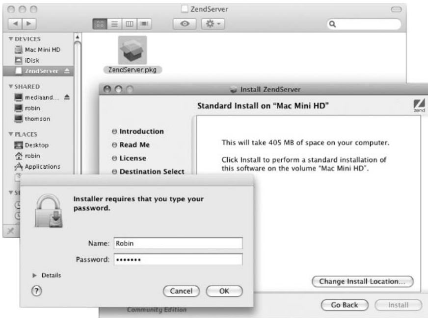
FIGURE 1-23 After a series of prompts, questions, and answers, enter your password to begin installation.
